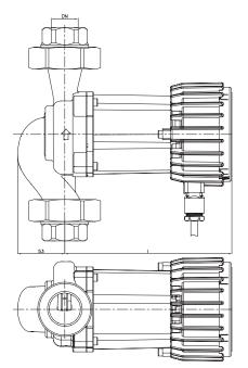
Flow Q up to 9 m<sup>3</sup>/h Pressure H up to 6 m Power 7 - 90 Watt Nominal pressure 10 bar
