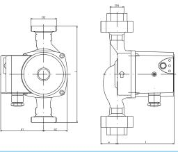
Flow Q up to 2,6 m<sup>3</sup>/h Pressure H up to 4 m Power 5 - 25 Watt Nominal pressure 10 bar
