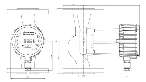
Flow Q up to 10 m<sup>3</sup>/h Pressure H up to 8 m Power 7 - 60 Watt Nominal pressure 10 bar
