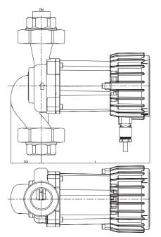
Flow Q up to 11 m<sup>3</sup>/h Pressure H up to 10 m Power 7 - 180 Watt Nominal pressure 10 bar
