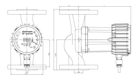
Flow Q up to 7,5 m<sup>3</sup>/h Pressure H up to 4 m Power 7 - 60 Watt Nominal pressure 10 bar
