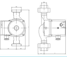
Flow Q up to 3,7 m<sup>3</sup>/h Pressure H up to 6 m Power 7 - 50 Watt Nominal pressure 10 bar
