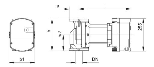
Flow Q up to 78 m<sup>3</sup>/h Pressure H up to 13 m Power 45 - 1600 Watt Nominal pressure PN6 or PN10
