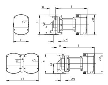
Flow Q up to 78 m<sup>3</sup>/h Pressure H up to 13 m Power 45 - 1600 Watt Nominal pressure PN6 or PN10
