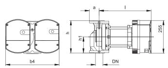
Flow Q up to 39 m<sup>3</sup>/h Pressure H up to 13 m Power 26 - 800 Watt Nominal pressure 6/10 bar
