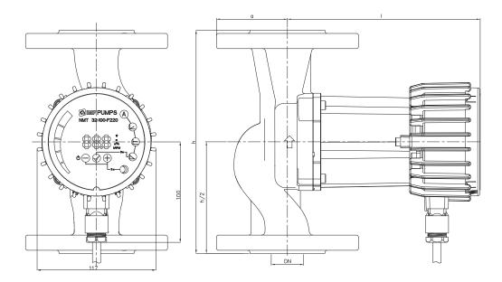
Flow Q up to 9 m<sup>3</sup>/h Pressure H up to 6 m Power 7 - 90 Watt Nominal pressure 10 bar
