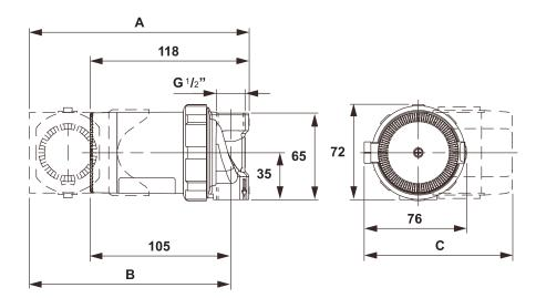
Flow Q up to 0,9 m<sup>3</sup>/h Pressure H up to 1,1 m Power 2 - 8 Watt Nominal pressure 10 bar
